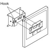
(2) By slightly lowering the LCD TV, you can hitch it on the hook.
